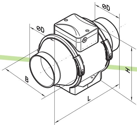
The Fanco TT series are designed for supply and exhaust ventilation of premises requiring high pressure and powerful airflow at a low noise level. The fans are compatible with round duct with models from 100mm to 315mm
