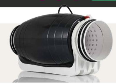
The all plastic construction includes inner perforations to reduce noise. The unit is wrapped in sound absorbing insulation which is contained within the black plastic housing.
