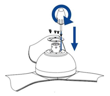
5. This fan comes with two rod options for installation - 125mm and 250mm. Select a rod to install (ensuring your fan is above the 2.1m required height). The rod installs with the 3 holes up (closest to the roof).
