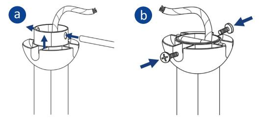
12. Hang the fan into hanging bracket. Align ball groove on hanging ball with ridge on hanging bracket. Ensure hanging ball sitting into hanging bracket correctly. If fan doesn't sit properly, hold the downrod and twist it until fan has been secured into hanging bracket.
