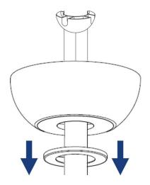
Place the canopy over the bracket, align the canopy holes with the screws and tighten. Clip it in to secure it onto the canopy.
