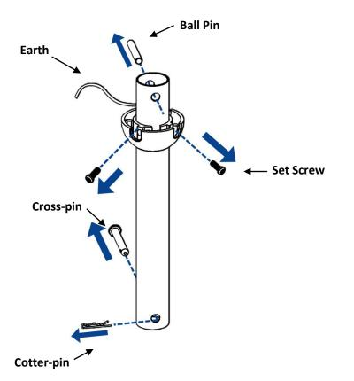
Feed the main motor wire and light wire plug (light models only) up through the inside of the downrod, then insert the downrod into the downrod holder. Gently push the cross-pin through the holes aligned with the base of the downrod holder and downrod.
