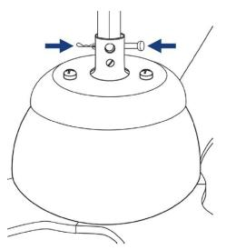
9. Snuggle the coupling cover down onto the top of the motor housing.
