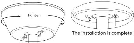
Rotate the canopy to align the holes and secure the canopy to the mounting bracket & tighten the screws
