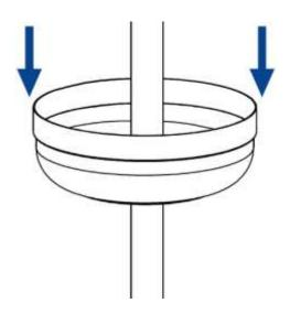
8. Place the hanging ball on top of the down rod and secure it using the ball pin and one screw.
