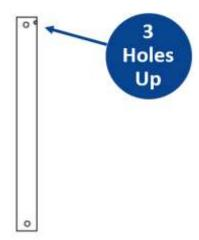
5. Feed the main motor wire and light wire plug (light models only) up through the inside of the downrod, then insert the downrod into the downrod holder. Gently push the cross-pin through the holes aligned with the base of the downrod holder and downrod. Insert cotter-pin into cross pin and secure downrod with two set screws.
