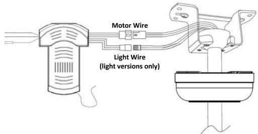
11. Place the canopy over the mounting bracket, align the canopy holes with the screws and tighten.
