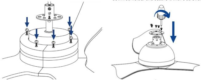
5. This fan comes with two rod options for installation - 125mm and 250mm. Select a rod to install (ensuring your fan is above the 2.1m required height). The rod installs with the 3 holes up (closest to the roof).
