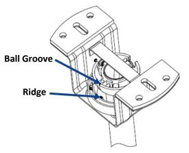
12. Place the receiver on top of the hanger ball and connect the wires. Connect power, receiver and the fan as per the electrical wiring diagram.
