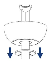
14. Place the canopy over the bracket, align the canopy holes with the screws and tighten. Clip it in to secure it onto the canopy.
