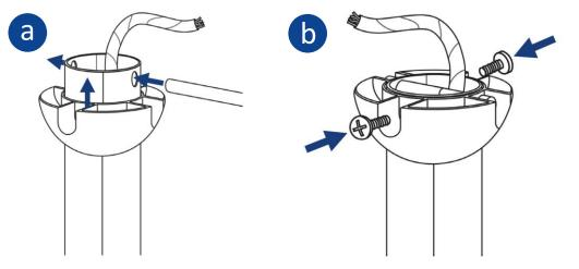
11. Hang the fan into hanging bracket. Align ball groove on hanging ball with ridge on hanging bracket. Ensure hanging ball sitting into hanging bracket correctly. If fan doesn't sit properly, hold the downrod and twist it until fan has been secured into hanging bracket.
