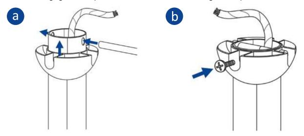
9. Hang the fan into hanging bracket. Align ball groove on hanging ball with ridge on hanging bracket. Ensure hanging ball sitting into hanging bracket correctly. If fan doesn't sit properly, hold the downrod and twist it until fan has been secured into hanging bracket.
