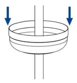
8. Place the hanging ball on top of the down rod and secure it using the ball pin and one screw.
