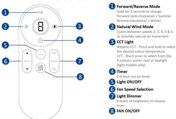
Once the Forward/Reverse is held for 3 seconds, the display will show alternating bars which will indicate the fans direction. When it moves from top to bottom the fan is in forward (summer mode). Bottom to top means reverse (winter mode).
