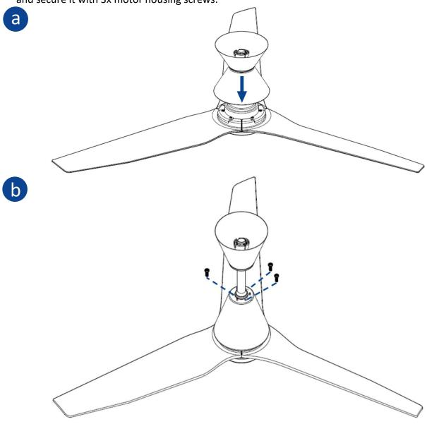
**MODELS WITH LIGHT** - Remove the three screws on the middle of the motor. Align the light kit with the screw holes on the motor housing and secure with screws. Connect the push plug wire attached on the light kit with the push plug attached to the motor.
