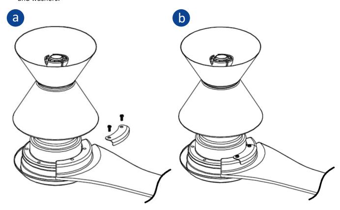
4. Once all blades are securely attached to the motor, simply slide the motor housing down into place and secure it with 3x motor housing screws.
