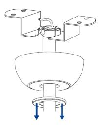
12. Place the canopy over the bracket, align the canopy holes with the screws and tighten. Clip it in to secure it onto the canopy.
