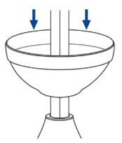
8. Place the hanging ball on top of the downrod and secure it with the ball pin and two set screws. **CAUTION**: Secure one screw through holes on the hanging ball and the downrod.
