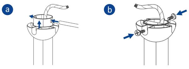
9. Hang the fan into hanging bracket. Align ball groove on hanging ball with ridge on hanging bracket. Ensure hanging ball sitting into hanging bracket correctly. If fan doesn't sit properly, hold the downrod and twist it until fan has been secured into hanging bracket.
