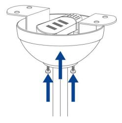
**MODELS WITHOUT LIGHT** - Place bottom plate to the bottom of the motor and screw it clockwise into motor shaft until it is secured. **IMPORTANT: DO NOT OVER TURN.**
