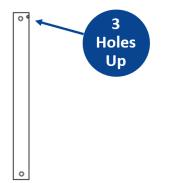
4. Feed the main motor and light wire (light version only) plug up through the inside of the downrod, then insert the downrod into the downrod holder.
