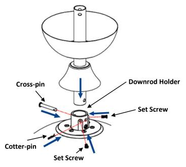
Snuggle the coupling cover down onto the top of the motor housing. Put the canopy through the downrod.
