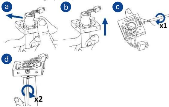
iii. Hang the fan into hanging and tighten it with 4 screws.
