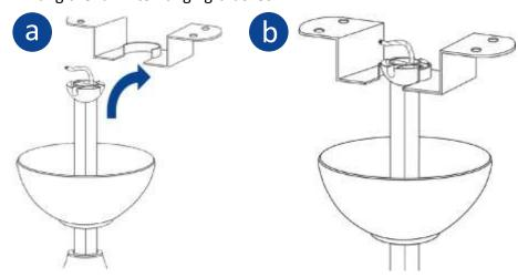
iii. Align ball groove on hanging ball with ridge on hanging bracket.
