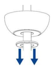
12. Place the canopy over the bracket, align the canopy holes with the screws and tighten. Clip it in to secure it onto the canopy.
