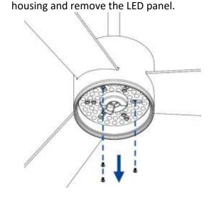
c. Remove the 3 screws from the light kit
