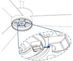
f. Align the diffuser to the bottom of the motor and rotate clockwise until it locks securely into place. **IMPORTANT: DO NOT OVERTURN**
