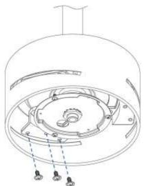
**MODELS WITH LIGHT** Remove the 3 light screws on the light plate.
