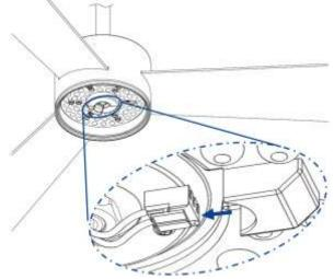
d. Align the new LED panel and secure with LED the mounting screws
