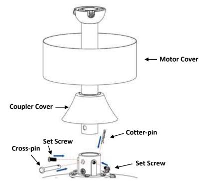
5. Snuggle the coupling cover down onto the top of the motor housing. **CAUTION: DO NOT** remove rubber gasket on top of the coupling cover.
