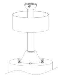
6. Remove the 9 blade screws from the bottom of the motor casing.
