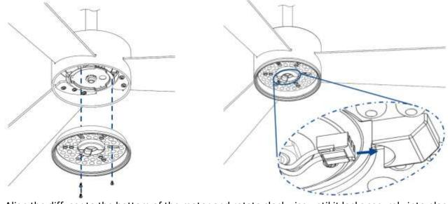
3. Align the diffuser to the bottom of the motor and rotate clockwise until it locks securely into place. **IMPORTANT: DO NOT OVERTURN**
