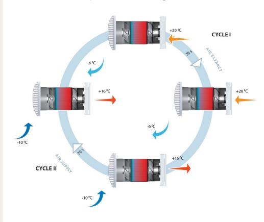
Decentralised heat recovery units are designed to **extract** and **supply**. In the first cycle warm, stale air is extracted from the room. As the warm air passes through the ceramic element, this component gets heated. The unit then commences cycle 2, clean air from the outside passes through the ceramic element, which heats the air before it enters the living space.
