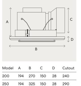
Minimum install depth on both models 220mm
